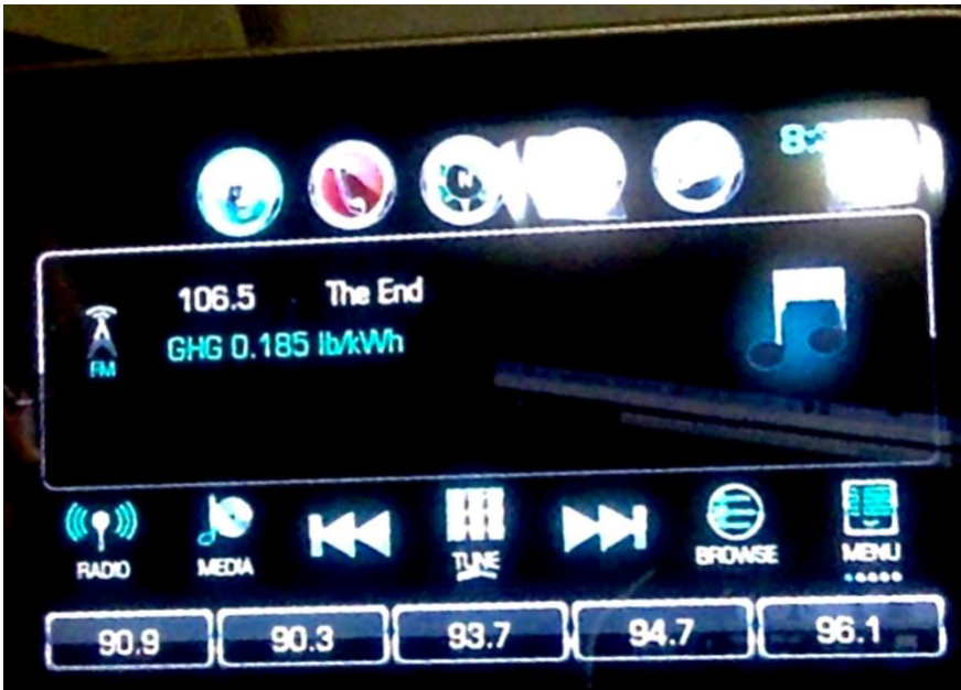
Figure 3. Broadcast of WattTime emissions data to an EV via KUDL Sacramento, March 12, 2021.
