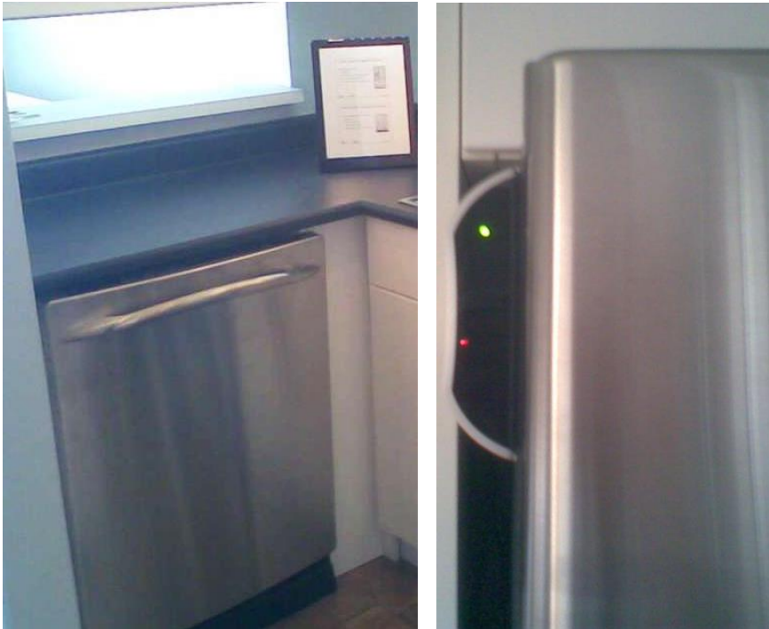
Figure 6. Pre-production Dishwasher and refrigerator (2008) responsive to FM broadcast
