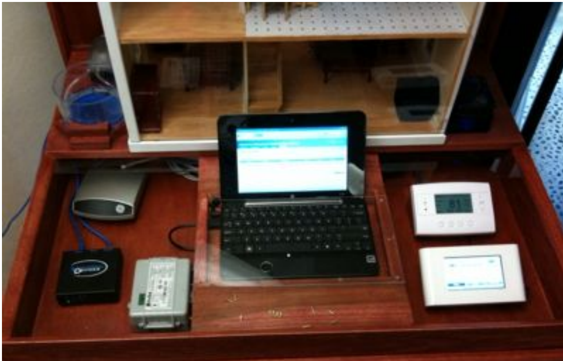
Figure 10. The residential OpenADR demonstration unit
