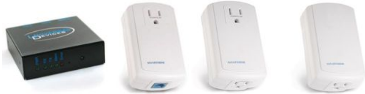
Figure 6. ISY-99i Controller with SmartHome PowerLinc Modem, LampLinc and ApplianceLinc modules
