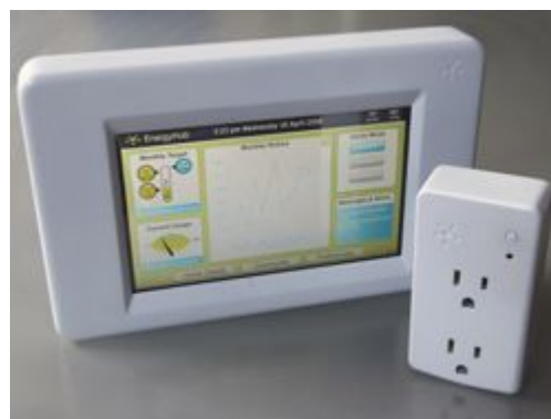
Figure 8. EnergyHub dashboard and Plug-load monitor
